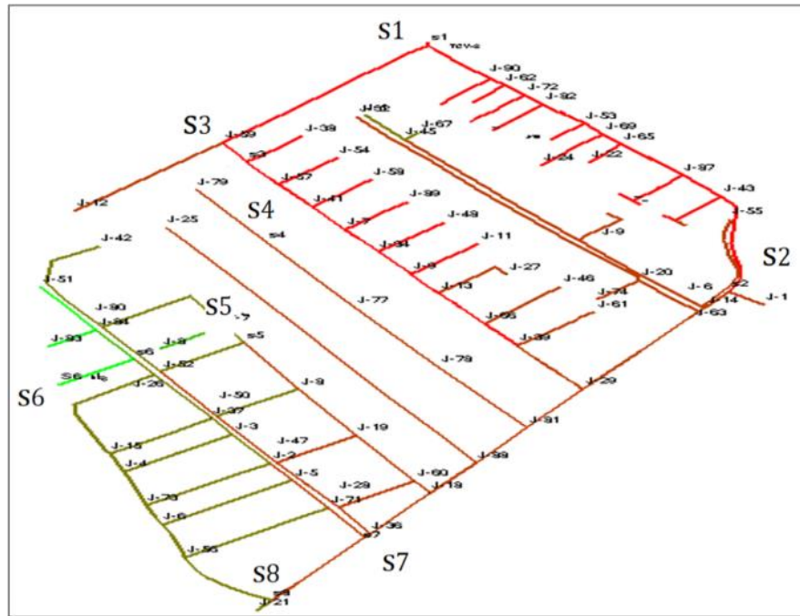
Figure 1. Hydraulic Model Layout of the Water Distribution Network Developed and Analyzed Using EPANET
